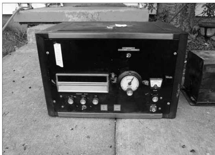
#5. Marsh's AZ-58 update in the 1970's with a solid state audio oscillator.
